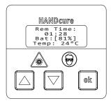
The exposure phase starts after 3 brief warning pulses. The preset time elapses. The exposure phase ends when the set time elapses
